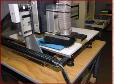
Once the data has been accumulated the blocker is set up and milled.
