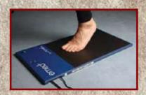
The TrueContour™ system comprises shape and pressure measurement devices (pictured above), operated by an easy-to-use graphical user interface through which the practitioner gathers, and then transmits, the patient data to Acor's central fabrication facility.
