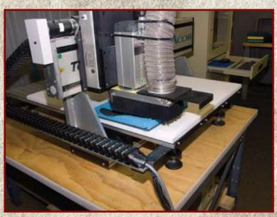
Once the data has been accumulated the blocker is set up and milled.
